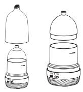
2.Fill the water tank with clean, cold or purified water. Water temperature should be around 6°C to 40°C. Do not pour water above the MAX scale level of the tank.
